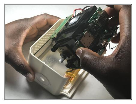
• Remove the inner components from the outer shell.
