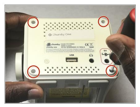
Remove the four 2mm screws with a Phillips screwdriver.
