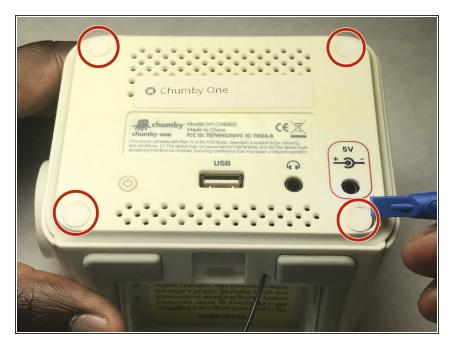
• Remove 4 self-adhesive plastic dots covering the screw holes.
