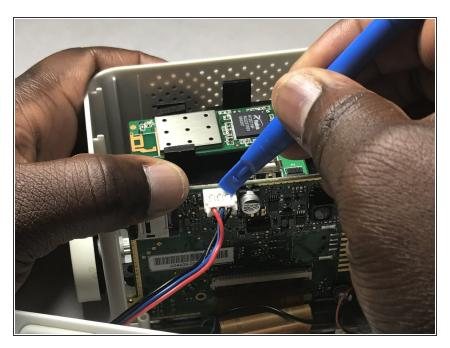
• Disconnect the battery connector from the motherboard with a plastic opening tool.
