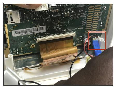
Disconnect the microphone connector from the motherboard with a plastic opening tool.
