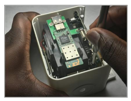
• Remove the four 6mm screws using a PH000 bit on the inner chassis.
