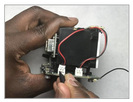
• Remove the speaker wire connector from the motherboard.
