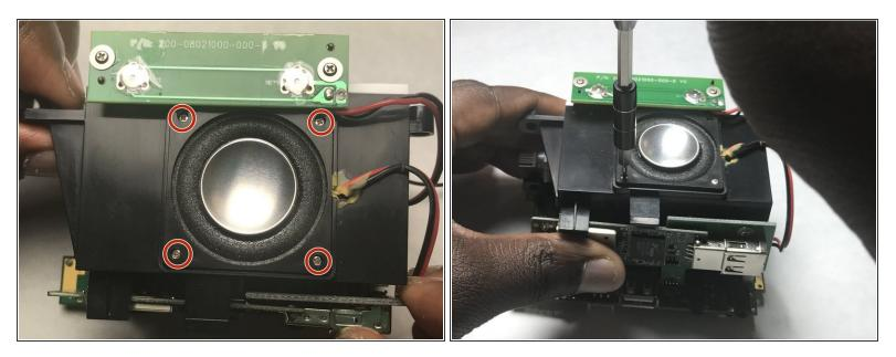
• Remove the four 5mm screws on the speaker base with a Phillips PH00 screwdriver bit.
