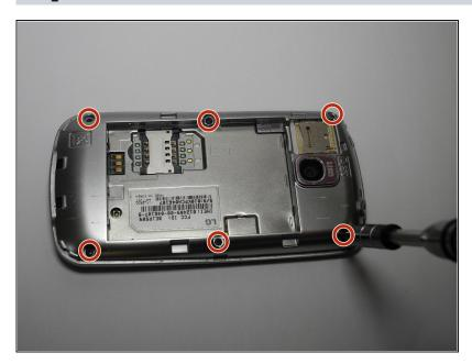
Use a J0 screwdriver to remove the 6 highlighted screws
