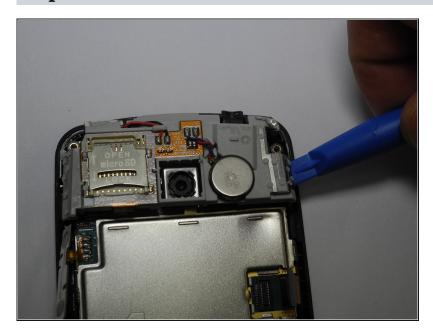
Remove SD card mount by inserting the plastic opening tool on the right side of the device to pop mount off
