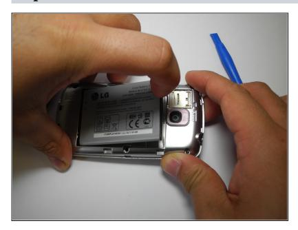
Remove the battery by pulling up on the battery using the indentation to the left of the camera lens
