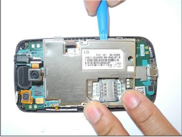
Remove metal panel by inserting plastic opening tool into the four retaining points and remove panel
