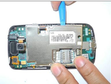
Remove metal panel by inserting plastic opening tool into the four retaining points and remove panel
