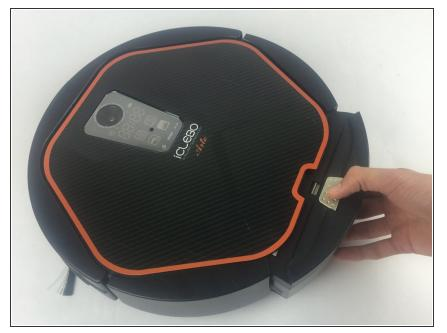
Remove the dust bin by gently pressing the silver button on top of the vacuum until the bin releases.
