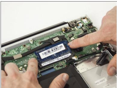
Press down and out on the topside of the clips holding the memory in place.
