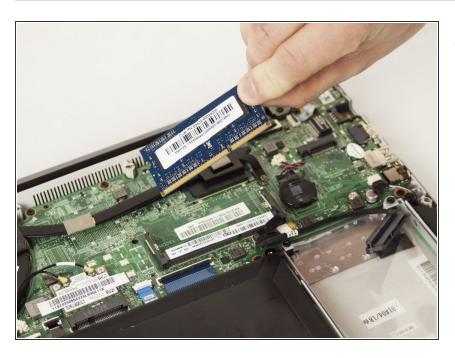
Once the clips are free, pull the topside of the memory up, and then remove it from the slot.
