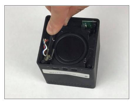
Using tweezers remove excess glue that may be covering the screw holes of the speaker's driver.
