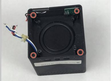
Remove the four 10mm screws from speaker's base.
