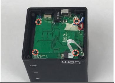
Unscrew the four 10mm screws from the motherboard.
