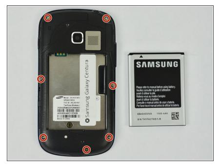
Find the positions of the seven screws on the back of the device.
