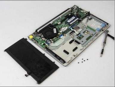
Once the battery is disconnected, lift up on the front of the battery and remove it from the laptop body.
