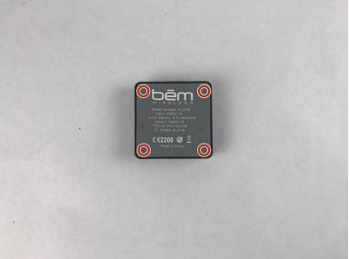
Use the J1 bit attached to the screwdriver to remove the four 10mm screws from the bottom of the auxiliary charging base.
