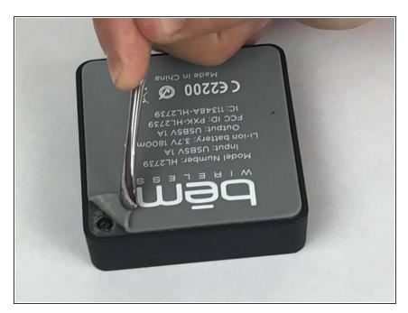
Peel the rubber cover back from the corner of the auxiliary charging base to reveal the screw.
