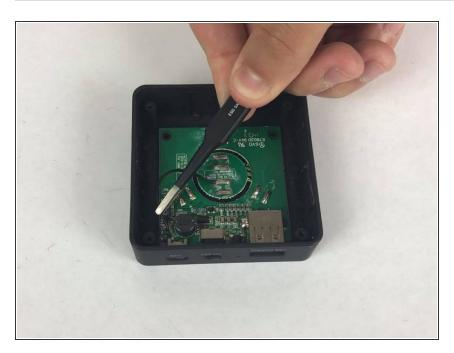
Using tweezers, remove the black wire from the motherboard
