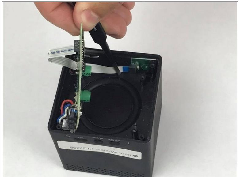
**⚠** Gently re-position the motherboard so you can access the bus wire connected to the speaker.
