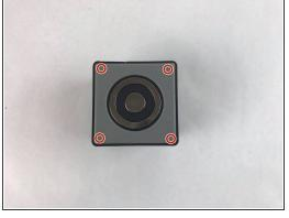
Use the J1 bit attached to the screwdriver to remove the four 10mm screws from the bottom of the speaker.
