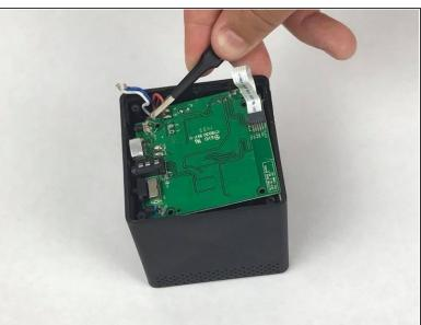
Using tweezers, remove the blue/white and red/black wires from motherboard.
