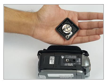
The tripod adapter can now be lifted out and replaced.
