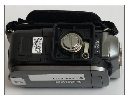
Locate the tripod adapter on the bottom of the camcorder.
