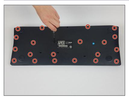
Unscrew the twenty black 4.5 mm Phillips #1 screws on the back of the keyboard.
