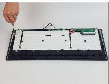
Unscrew the two silver 4.5 mm Phillips #1 screws and the seven 5.0 mm Phillips #1 screws that deter the plastic panel from removal.
