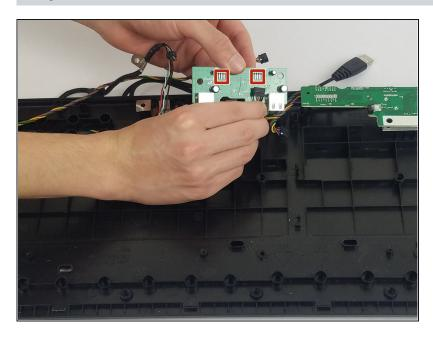
Unplug the wires and remove the USB port connector.
