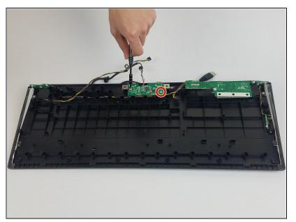
Unscrew the two 4.5 mm silver Phillips #1 screws that hold the USB port connector.
