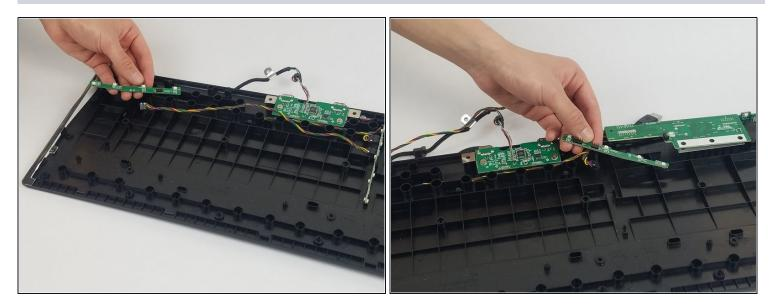
Remove the LEDs.
