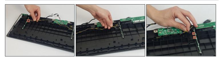
Unplug the wires connected to the LEDs.
