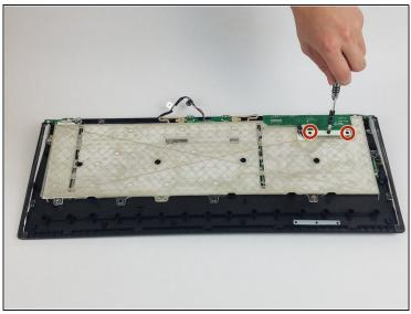
Unscrew the two silver 4.0 mm Phillips #1 screws and the three black 6.5 mm Phillips #1 screws holding the silicone sheets.
