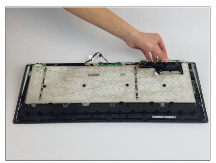
• Flip the chip slightly in order to remove the sheets.
