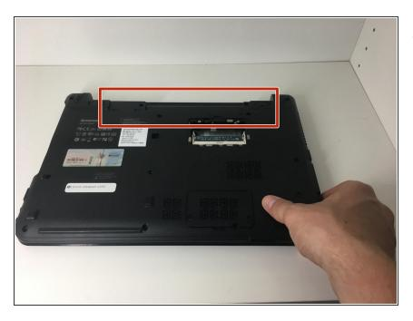
Remove the unlocked battery.
