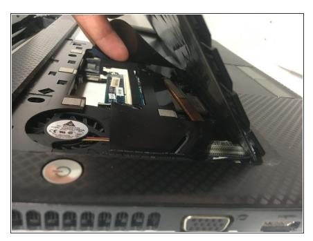
Disconnect the wire connecting to keyboard to the laptop.
