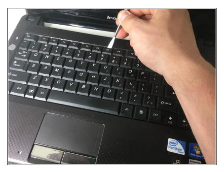
Use the spudger to pry the top of the keyboard out.
