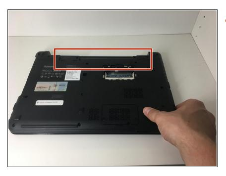
Remove the unlocked battery.
