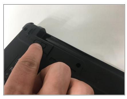
On the top left of the laptop there is a switch. Make sure it's pushed in the unlocked position.
