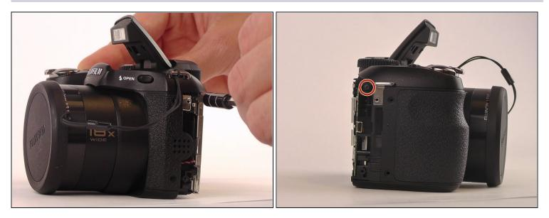
• Remove the 4 mm screws from the left and right sides of the camera with the JIS #1 screwdriver.
