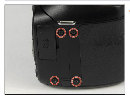
Unscrew the four 4mm screws on the right-hand side of the camera with the JIS #1 screwdriver.
