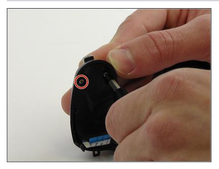
Remove the two 2 mm screws underneath the plate with the Phillips #000 screwdriver.
