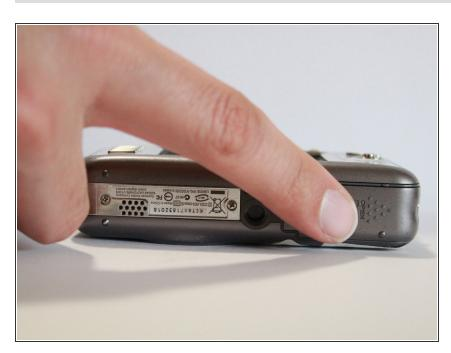
With your finger, slide the battery cover in the direction of the open arrow.
