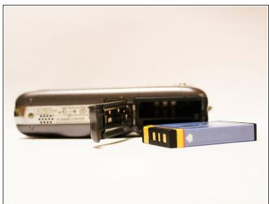
• Gently push the battery down until a click is heard. Battery should release and be lifted out of slot.
