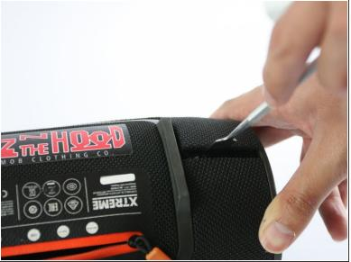
• Use the metal spudger to gently pry and lift the edge of the seam. The cover is held in place with plastic snaps that will make a popping noise when disengaged. !!Start with the back half, this will expose TWO Screws that need to be removed before lifting the front half.
