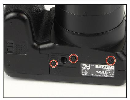
Unscrew the three 4mm screws on the bottom of the camera with the JIS #1 screwdriver.
