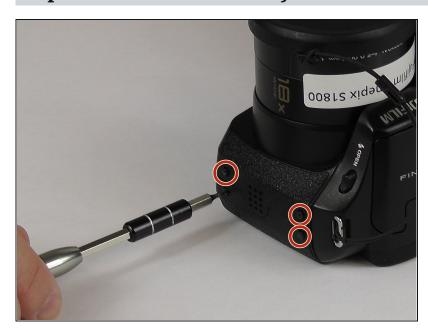
Unscrew the four 4mm screws on the left-hand side of the camera with the JIS #1 screwdriver.
