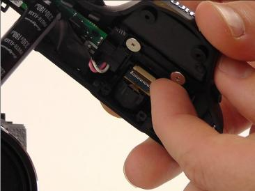
• Switch the lever to disconnect the micro strip that connects the top plate. **Do not** rip the micro strip.
