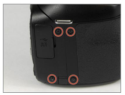
Unscrew the four 4mm screws on the right-hand side of the camera with the JIS #1 screwdriver.
