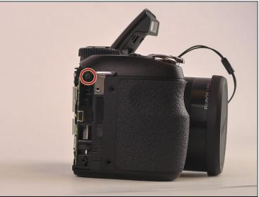
• Remove the 4 mm screws from the left and right sides of the camera with the JIS #1 screwdriver.
