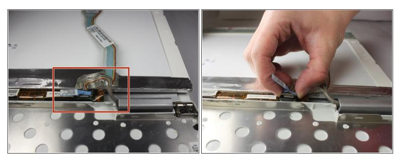
Remove the next connection by pressing the two metal sides towards the middle. Then gently pull
