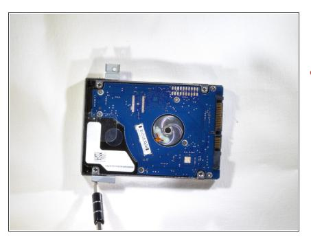
• To remove the hard drive mounting bracket, locate the screws holding it on. There is one, 4mm long M2 screw on each of each on the long edges of the drive, and remove them. This will free the drive from the bracket. The bracket is needed to put the new drive back into the computer.
