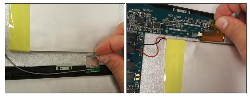
Remove the two pieces of tape on the battery.
