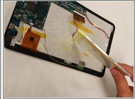
Pry off the battery with a plastic opening tool.
