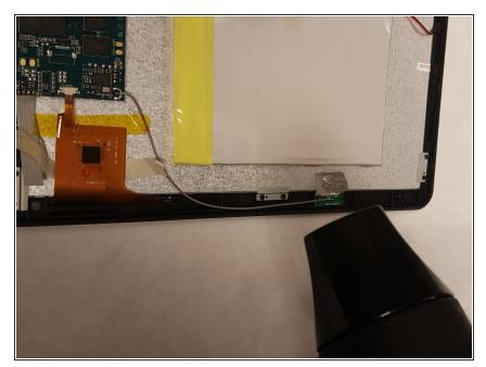
Apply heat around the edges of the battery with a hair dryer.
