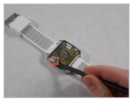
Disconnect the ribbon cable on the left side of the motherboard by using a spudger.
