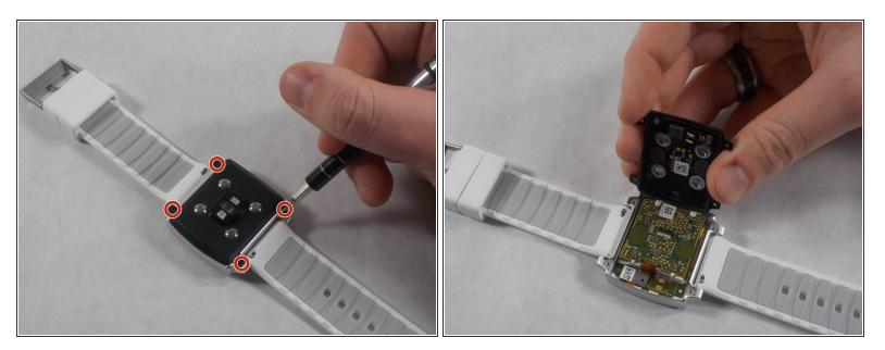
Remove the four base screws using a size 2 TORX screwdriver to separate the back plate from the frame.
