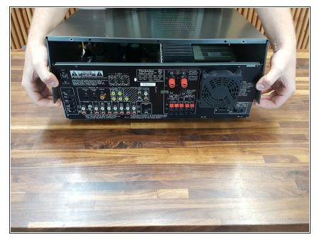
Lift up the device housing carefully. It helps to start at the rear bottom corners and pull out a little. Make sure that once the rear edges of the housing are free that you lift the front edge straight up to separate it from the front display assembly.
