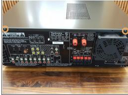
Remove four case screws on the left and right sides, then remove two screws at the top of the back side.
