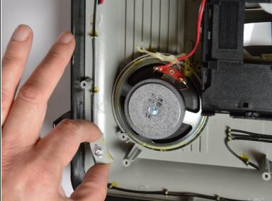
Be sure to unscrew (3 mm) the two plastic brackets on each speaker, use iOpener or heat gun they are glued onto speakers, please do not discard.
