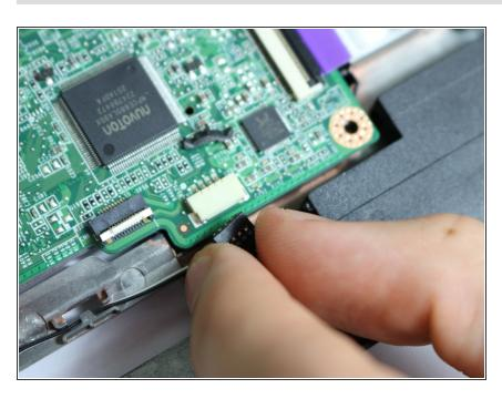
Disconnect the speakers from the motherboard by carefully pulling the adapter away from the center of the device.
