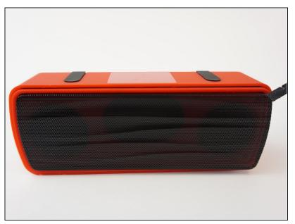
• Slide the spudger along the separation between the grate and the base of the speaker to loosen the grate. Do this to the entire perimeter of the speaker.
