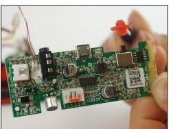
• Using tweezers, detach the power button from the mother board.
