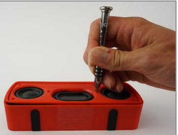
• Remove the six 3mm screws using the J00 JIS screw bit. This will require a long, narrow screwdriver.
