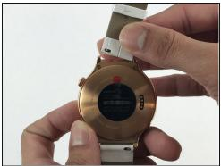
• Use the Flex Extension to push the spring to the right. This will release the strap from the watch head.
