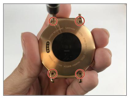
Locate the 4 T3 screws in the back of your watch, and use the T3 Torx Screwdriver to unscrew them.
