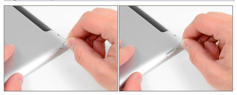
• Use a SIM eject tool or an uncoiled paperclip to eject the SIM tray.
