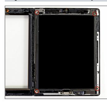
Remove the four 2 mm Phillips #00 screws securing the LCD to the aluminum frame.
