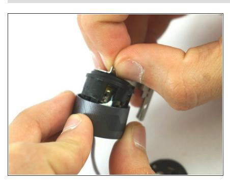
Separate the camera from its casing.
