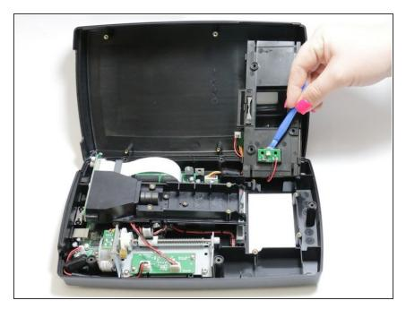
Lodge the plastic opening tool underneath the bulb casing. Using some upward force, pop the bulb off the casing.
