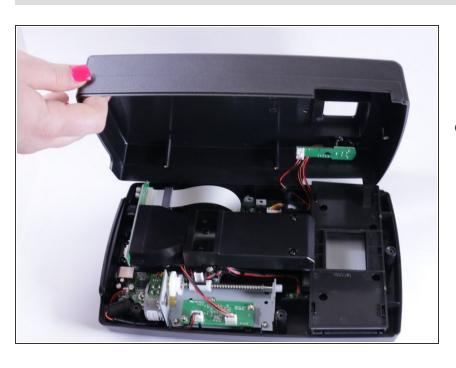
Now that the screws have been removed, carefully but firmly open up the device at the seam until it is presented as shown.
