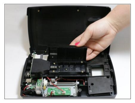
Now grab the plastic cover you just removed screws from and gently remove it from the device.
