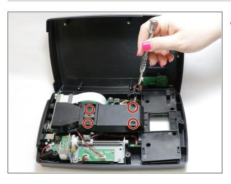
Use the same J0 screwdriver to remove the following 3 screws that are 7mm x 6mm.
