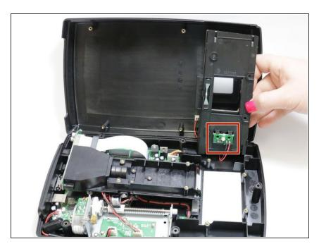
You may now pick up the plastic covering you removed screws from in Step 3 with ease revealing the bulb.
