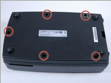
Start by removing the 5 screws that are 5mm x 9mm located on the bottom of the device with a J1 screwdriver.
