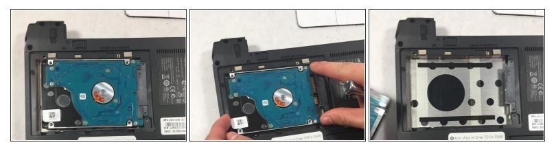
• Remove the hard drive by sliding it to the left and pull it out.
