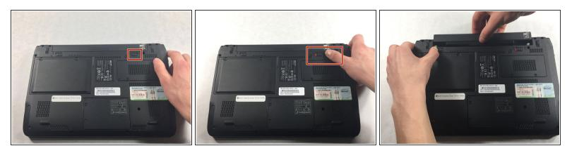
Unlock the right side of the battery by sliding the battery lock to the right. Then slide the left lock to the left and remove the battery.
