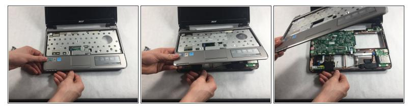
• Separate the front panel from the back panel, by sliding your thumb nail between them.
