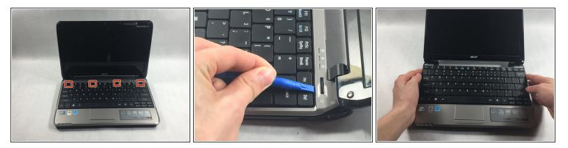
• Use the plastic opening tool to push in each of the four clips and carefully lift the keyboard.
