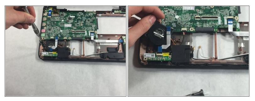
• Unscrew the Phillips #0 (M2-L2.5 mm) screw from the fan, and remove the fan.
