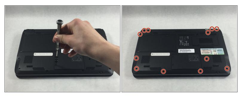
Use the screwdriver to remove Phillips #0 (M2-L5 mm) screws
