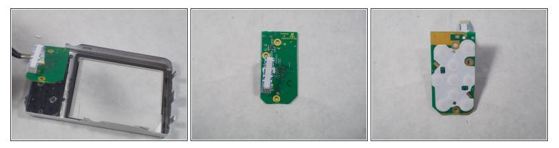
• Lift the chip with tweezers to remove it from the other remaining components.
