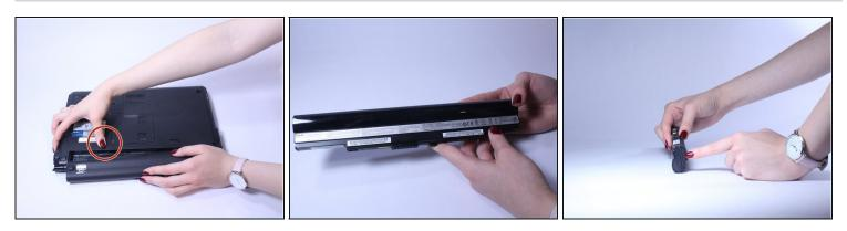
• Slide the button marked with an arrow to the left. The battery should now unclick. Slide the battery away from the laptop to remove it.
