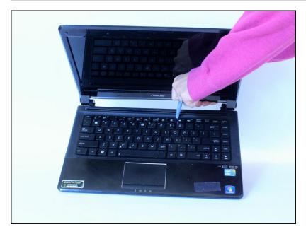
Insert a plastic opening tool or a flat-head screwdriver between the laptop body and the keyboard.
