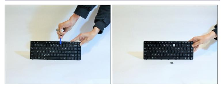
• Gently insert the plastic opening tool between the key cap and the hinge. Slowly push the screwdriver up. The key should pop up easily.
