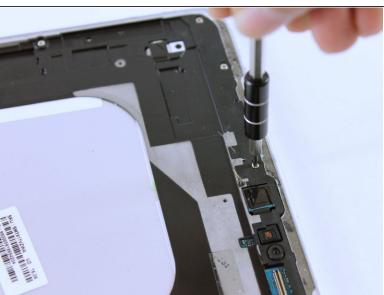
Remove all seventeen 3 mm screws using a PH000 Phillips screwdriver.
