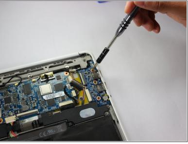
Unscrew four 1.2mm Phillips screws using Phillips #1 screwdriver.
