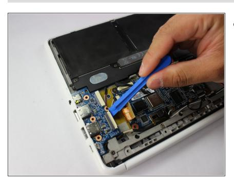
Using the plastic opening tool remove the audio port from the back panel.
