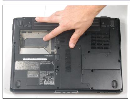
Remove the hard drive by pulling up on the black tab on the right side of the hard drive.
