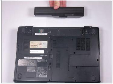
• Push the battery forward to eject it from the laptop.
