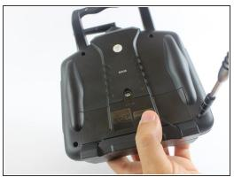
Remove the six 8.8 mm screws located on the back panel of the controller using a Phillips 000 screwdriver.
