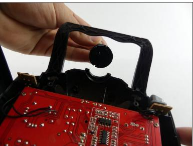
• Then, pull the antenna up and out of its location.
