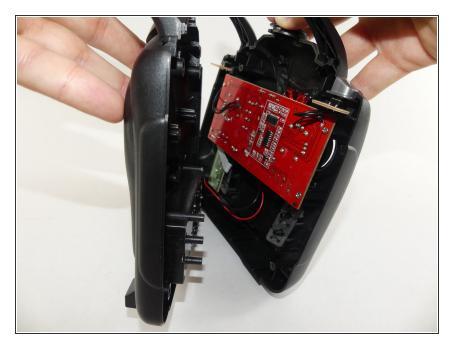
Carefully lift off the back panel of the controller.
