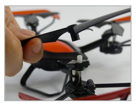
Carefully pull up the rotor blade.
