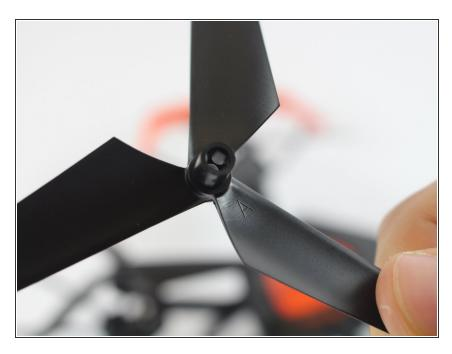
When putting the new blade in, align the new rotor blade with rotor blade shaft and make sure they have matching letters.
