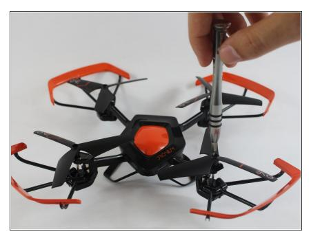
Remove the 6.0mm rotor blade screw using a Phillips 000 screwdriver.
