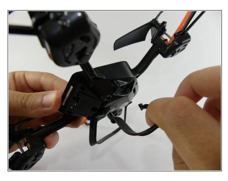
Once the inside screws are removed, carefully pull off the one of the landing gear legs. Repeat this step for the other leg. To reassemble your device, follow these instructions in reverse order.
