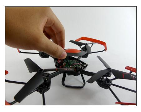
Once all of the screws are off, lift off the top of the drone.
