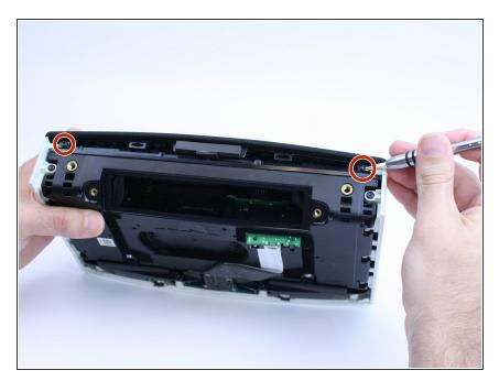
Remove the two torx screws holding the speaker grill in place.
