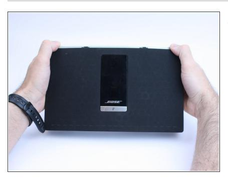
Grip the sides of the device and push the speaker grill down and out.
