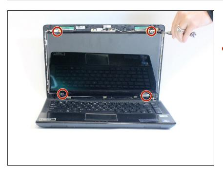
Unscrew the four 3 mm screws that hold the mounting brackets for the screen to the backing.
