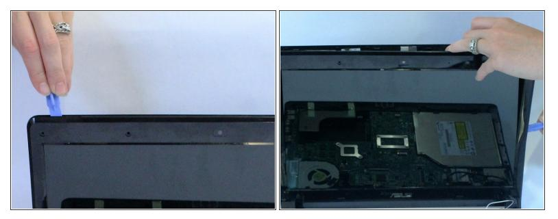
Next, completely remove the bezel using a plastic opening tool to work your way around while gently prying it from the LCD. If it does not come off with a moderate amount of force check that you did not miss any screws.
