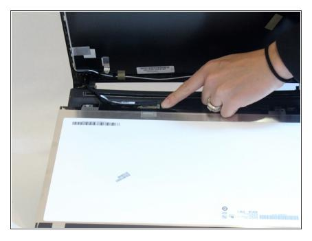
Gently lay the screen on the keyboard and remove the tape over the connection. You can then disconnect the screen.
