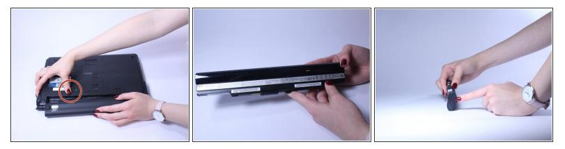
Slide the button marked with an arrow to the left. The battery should now unclick. Slide the battery away from the laptop to remove it.
