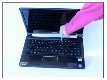
Insert a plastic opening tool or a flat-head screwdriver between the laptop body and the keyboard.
