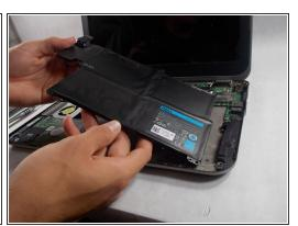
Remove the screws surrounding the battery and unplug the cable in the top left corner to then remove the battery.
