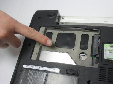
Using your fingers, open and remove the access door from the laptop, exposing the hard drive underneath.
