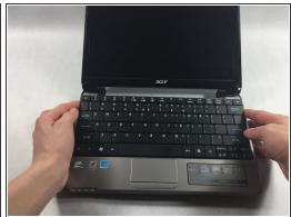
• Use the plastic opening tool to push in each of the four clips and carefully lift the keyboard.
