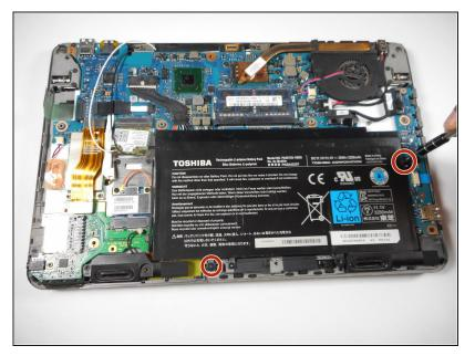
Use the screwdriver to remove the two 3.4 mm screws highlighted.
