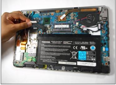
Remove the black cable from the connector. Pull in the same direction as the black wiring runs.
