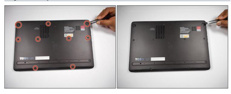
Use tweezers to remove the nine rubber grip pads on the back panel of the laptop.
