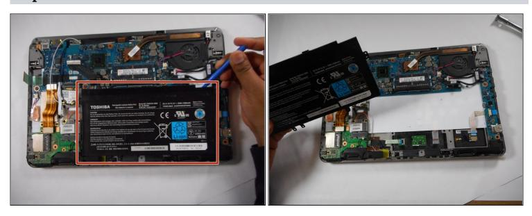
• Lift and remove the battery from the device with the iFixit opening tool.
