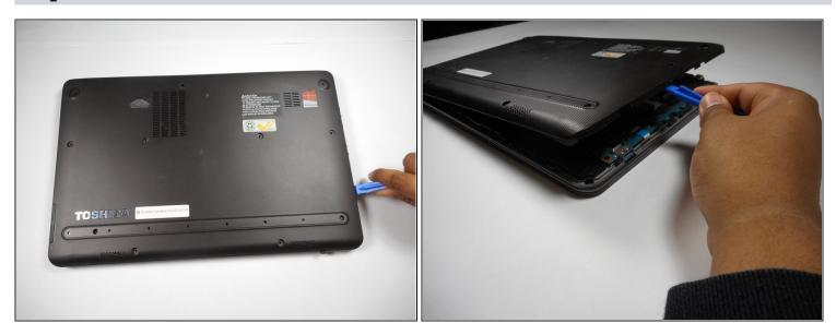
• Remove the back panel by inserting the plastic opening tool into the seam of the laptop and pushing downwards.
