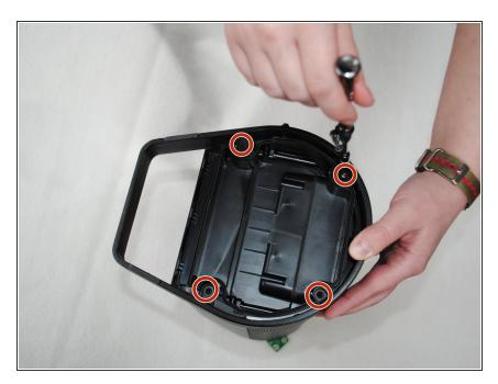
Using a Phillips # 1 screwdriver, remove the four 1.1 sm screws attaching the metal ring to the bottom of the device.
