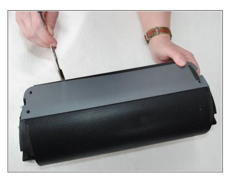
Using the metal spudger, pry off the side panel. Repeat this step on the other side panel.
