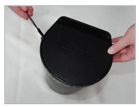
Using the metal spudger, remove the outer cap from the top of the device.
