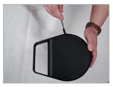
Using the metal spudger, remove the cap from the bottom of the device.
