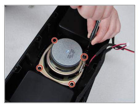
Using a Phillips #1 screwdriver, remove the four 1.2 cm pan head screws surrounding the speaker.
