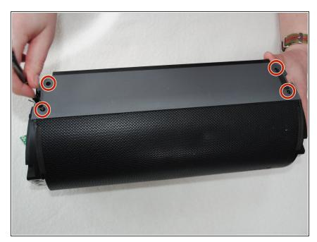
Using a Phillips # 1 screwdriver, remove the four 1 cm screws from the outside panel. You will do this for each panel; it does not matter which side you start with.
