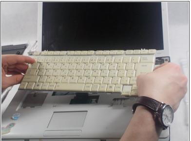
Pop out the black plastic tab on either side of the ribbon cable. Holding the cable on each side, detach from laptop.
