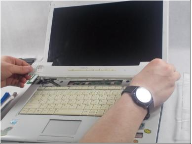
Run the blue plastic opening tool underneath the media bezel and gently pry from the front panel.
