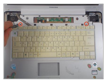
Using the #J0 bit, remove the two 3.1 mm screws securing the top of the keyboard.
