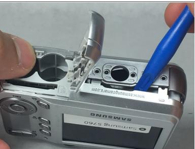
Use the plastic opening tool to open pry open the back case, following alongside the edge of the case if need be.
