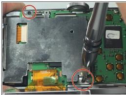
Under the LCD screen, remove the metal plate by removing the two 3mm screws holding it in place.
